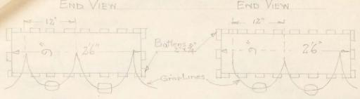
Buoyant Apparatus for 12 persons has a single metal air case 4:0" x 2:6" x 9".
